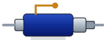
Mono-Strand Jack 20–30 t · 200 mm stroke
